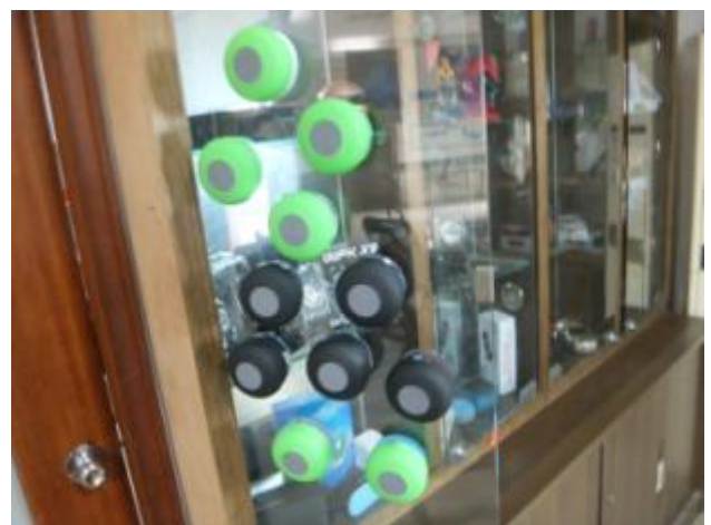
Suction function/endurance test on flat glass over 4hrs
